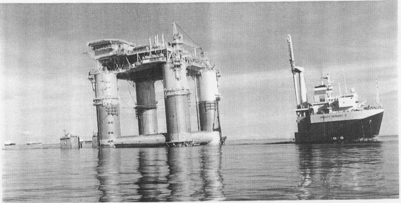
Figure 5 TLP lifted out of water with substantial trim by stern
